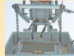
Heavy 1800 kgs Lift, suitable for heavy implements and tipping trailers with higher loads
