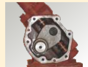
Recirculating Ball type Steering prevents transmission of shocks to the steering wheel.
