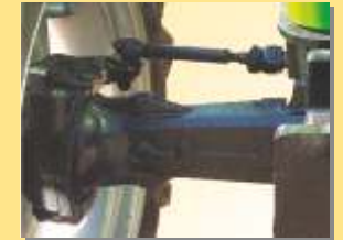
Heavy Duty Front Axle (4WD)/ Power Steering
