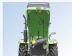
Aerodynamic Design- Easy approach for daily checkup like coolant level, air cleaner etc.
