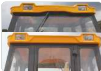
Front and rear canopy work lamps for improved visibility and ease of operation
