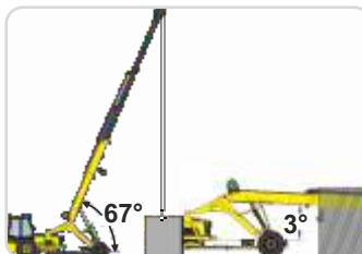
Luffing angle range: -3° to +67° for better safety and stability
